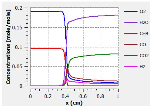
Main concentrations of stoichiometric CH<sub>4</sub> + air flame at standard conditions (298 K, 1 atm).
