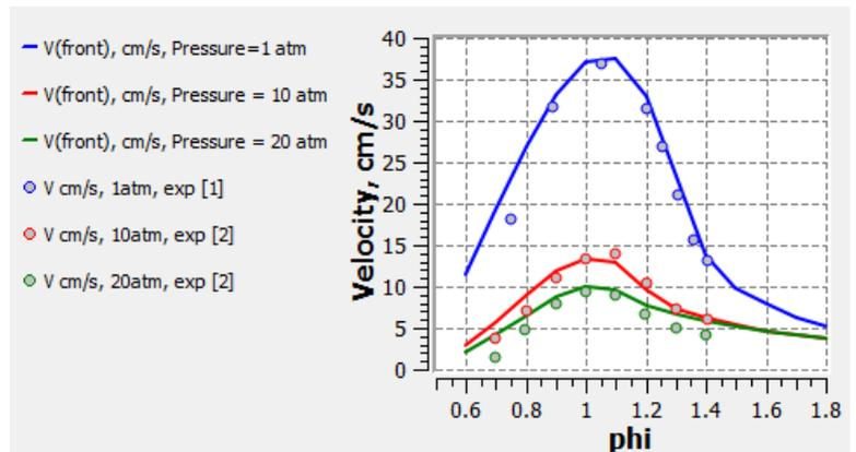
Laminar burning velocities of CH<sub>4</sub> + air flames at temperature 300 K and pressures 1, 10, 20 atm for  $\phi = 0.6- 1.8$ .
