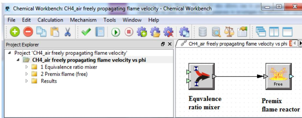
The first reactor **Equivalence Ratio Mixer** calculates composition of initial mixture at given  $\phi$ . The mixture CH<sub>4</sub>-air is inputted in this reactor - **Input Stream 1** - Fuel (CH<sub>4</sub>), **Input Stream 2** – oxidizer (air). This model requires kinetic mechanism. In this case the mechanism GRIMech-3.0 is taken. The Mechanism is loaded from KintechDB database, which is tightly integrated with Chemical Workbench.
