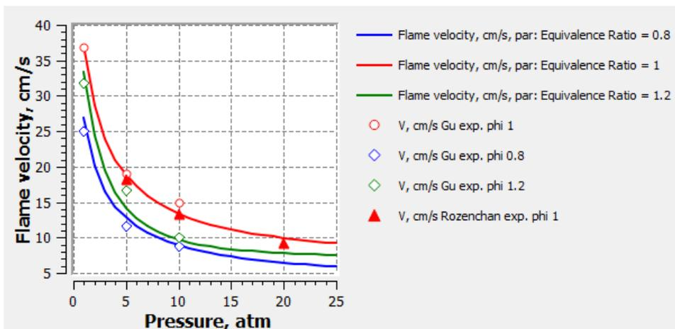
Laminar burning velocities of  $\text{CH}_4 + \text{air}$  flames as a function of pressure for fixed equivalence ratios 0.8, 1, 1.2 at temperature 300 K.
