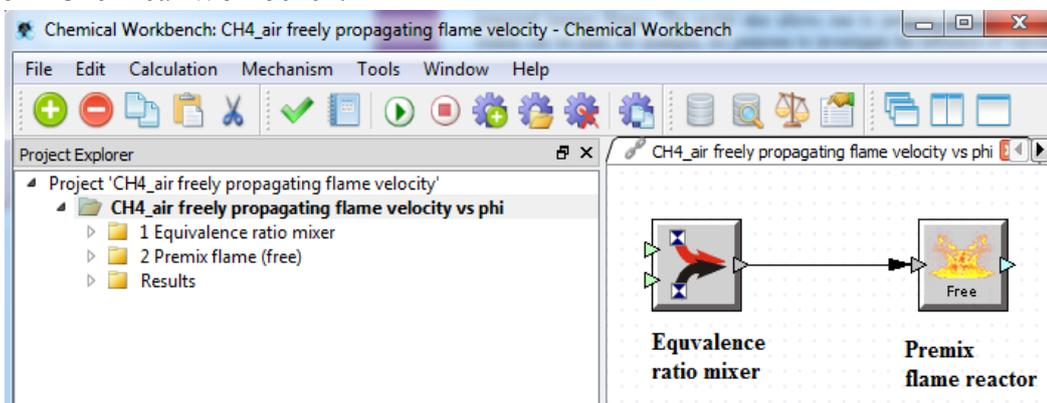
The first reactor **Equivalence Ratio Mixer** calculates composition of initial mixture at given  $\phi$ . The mixture of CH<sub>4</sub>-air is inputted in this reactor - **Input Stream 1** - Fuel (CH<sub>4</sub>), **Input Stream 2** – oxidizer (air). This model requires kinetic mechanism. In this case the mechanism GRIMEch-3.0 is taken. The Mechanism is loaded from KintechDB database, which is tightly integrated with Chemical Workbench.
