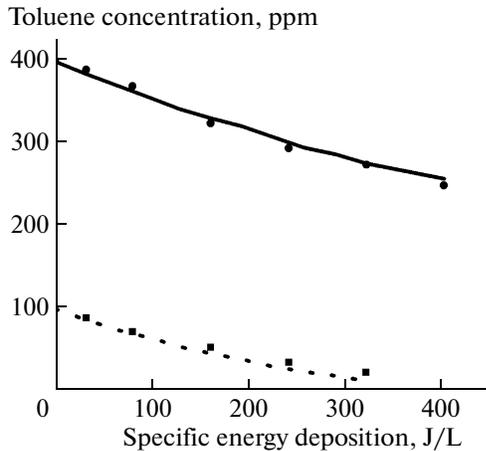
**Fig. 1.** Dependence of the toluene concentration at the reactor output on the specific energy deposition at  $[\text{C}_6\text{H}_5\text{CH}_3]_0 = 100$  ppm (squares) and 400 ppm (circles) for  $T = 323$  K. The symbols show the experimental data [9], and the solid and dashed curves are the simulation results for 400 and 100 ppm, respectively.
