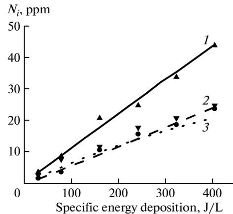
**Fig. 3.** Dependence of the concentration of by-products at the reactor output on the specific energy deposition at  $[C_6H_5CH_3]_0 = 400$  ppm and  $T = 323$  K: (1)  $C_2H_2$  (triangles and solid curves), (2) HCN (inverted triangles and dashed curves), and (3)  $CH_4$  (circles and dotted curves). The symbols show the experimental data [9], and the curves show the simulation results.
