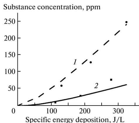
**Fig. 11.** Dependence of the (1) carbon monoxide CO and (2) carbon dioxide  $CO_2$  concentration at the plasma-chemical reactor output on the specific energy deposition in the gas mixture  $N_2 : O_2$  at the initial toluene concentration  $[C_6H_5CH_3]_0 = 400$  ppm, oxygen concentration  $[O_2] = 1.5\%$ , and gas temperature  $T = 323$  K. The curves show the simulation results, and the symbols show the experimental data [9].
