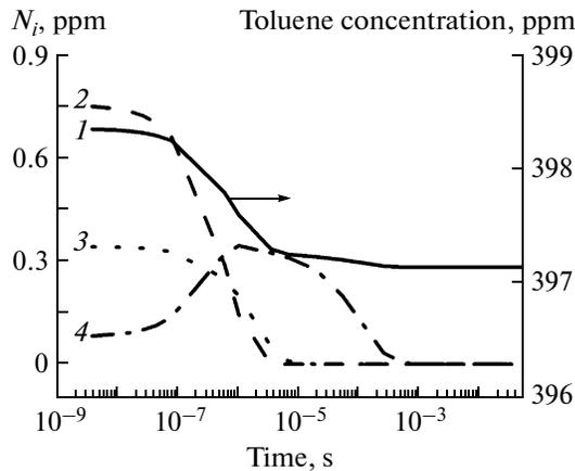
**Fig. 2.** Calculated temporal dynamics of toluene and active nitrogen components in the postdischarge stage of the second current pulse at the initial toluene concentration is  $[C_6H_5CH_3]_0 = 400$  ppm, gas temperature  $T = 323$  K, and specific energy deposition  $Q = 3.25$  J/L: (1) toluene, (2)  $N_2(A^3\Sigma_u^+)$ , (3)  $N_2(a^1\Sigma_u^-)$ , and (4) H.
