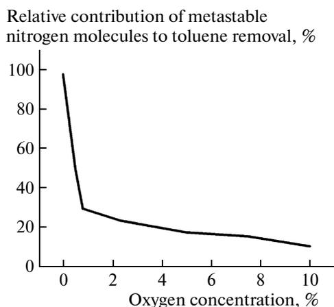
**Fig. 10.** Relative contribution of metastable  $N_2(A^3\Sigma_u^+)$  and  $N_2(a^1\Sigma_u^-)$  nitrogen molecules to the total toluene removal as a function of the oxygen concentration at the initial toluene concentration  $[C_6H_5CH_3]_0 = 400$  ppm and gas temperature  $T = 323$  K.
