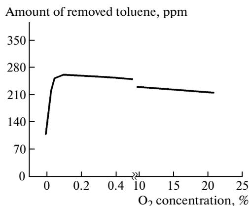
**Fig. 5.** Dependence of the toluene removal efficiency on the oxygen content in the gas mixture at the initial concentration  $[C_6H_5CH_3]_0 = 400$  ppm, gas temperature  $T = 323$  K, and specific energy deposition  $Q = 325$  J/L.
